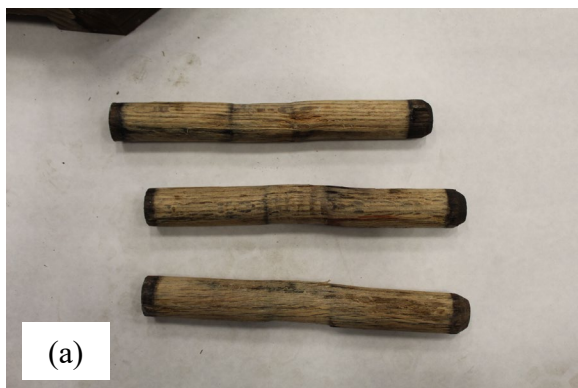
Fig. 4.13. Durability test specimen 3D: (a) peg bending, and (b) tenon failure.
