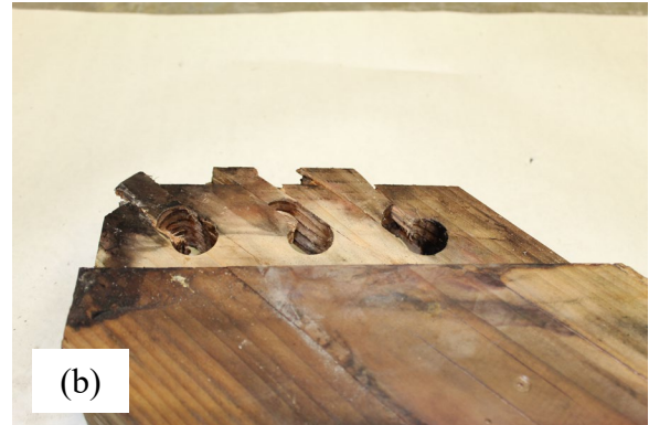
Fig. 4.11. Durability test specimen 2U: (a) peg bending, and (b) tenon failure.
