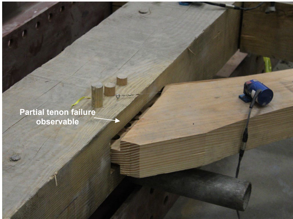
Fig. 3.11. Tenon failure in the right brace-beam connection.
