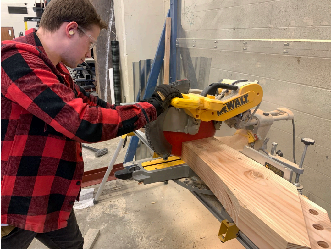
Fig. 4.2. Dividing newly manufactured brace for connection specimens.
