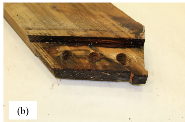
Fig. 4.13. Durability test specimen 3D: (a) peg bending, and (b) tenon failure.
