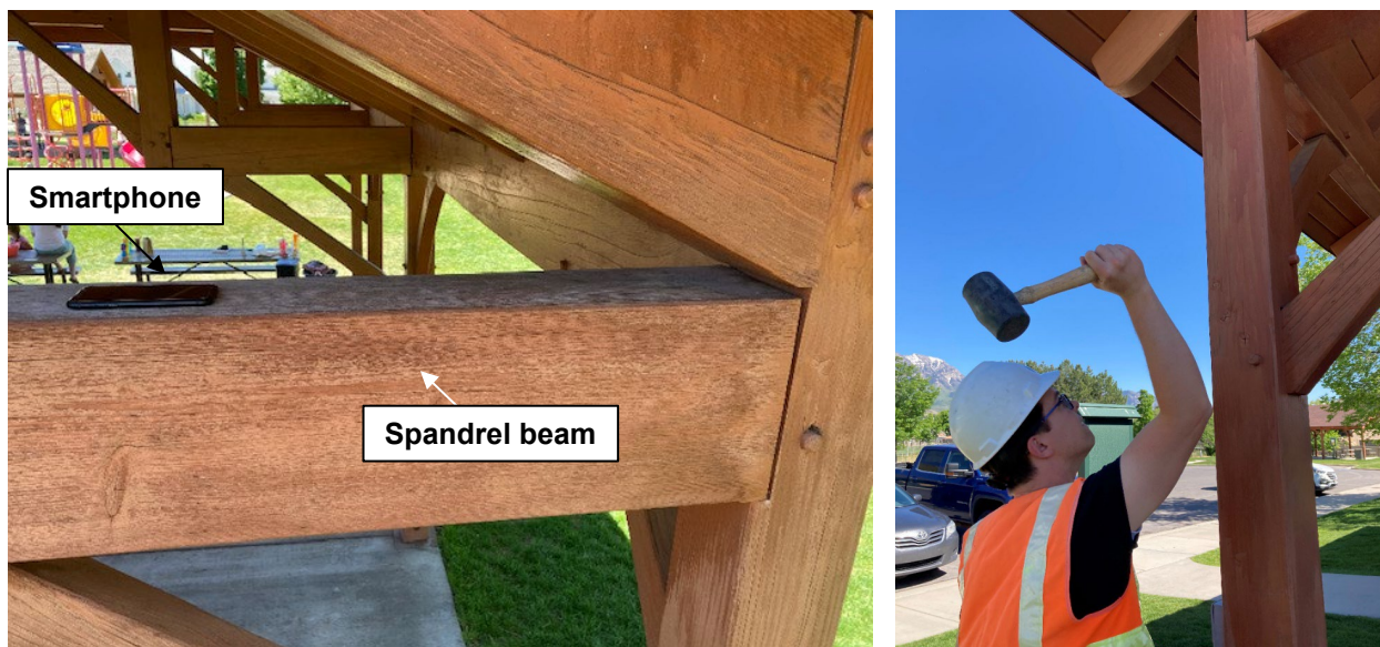
Fig. 5.2. Vibration test: (1) placement of smartphone, and (b) mallet strike.
