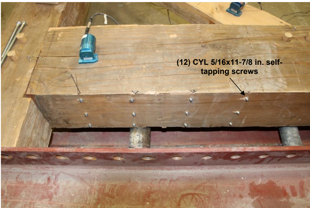
Fig. 3.18. Lag screws inserted in the top beam face to the right of the brace.
