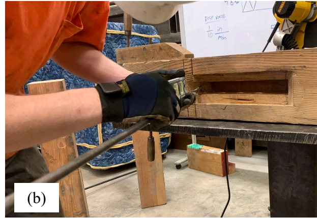
Fig. 4.3. Modification of connection details: (a) beveling out, and (b) boring bit insertion.
