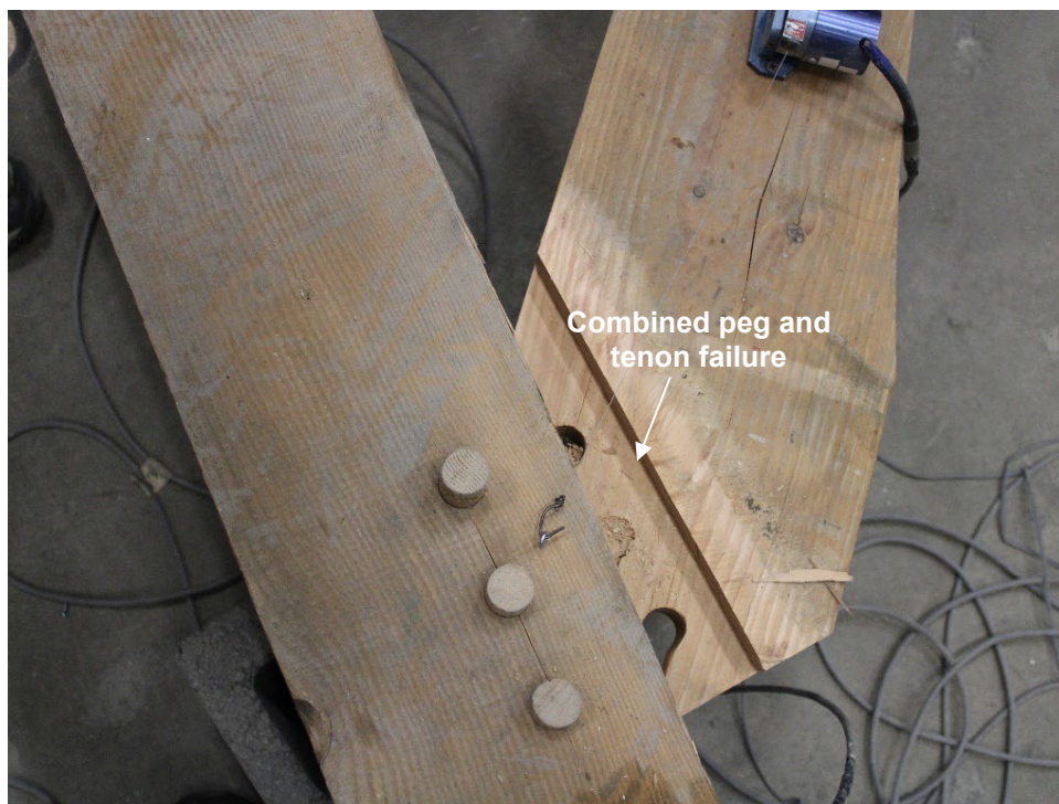
Fig. 3.12. Tenon failure in the right brace-beam connection.
