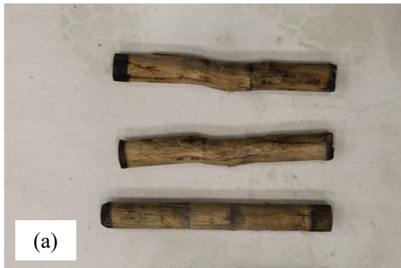
Fig. 4.12. Durability test specimen 3D: (a) peg bending, and (b) tenon failure.
