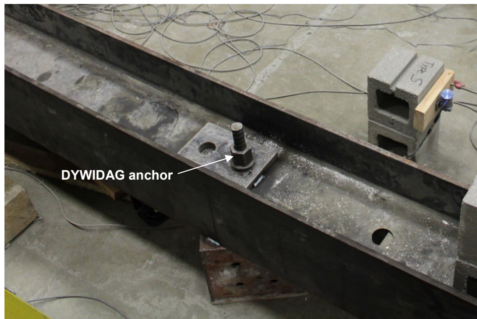
Fig. 3.5. DYWIDAG Anchors securing the support beam to the floor.
