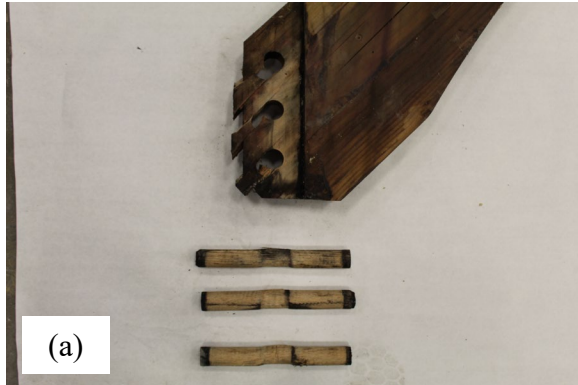
Fig. 4.11. Durability test specimen 2U: (a) peg bending, and (b) tenon failure.
