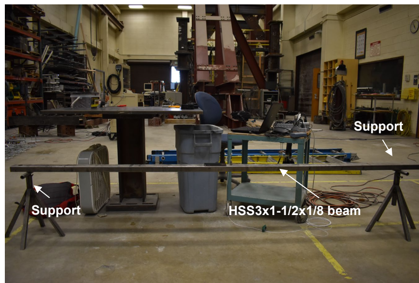
Fig. 5.12. Simply supported HSS beam for a vibration test.
