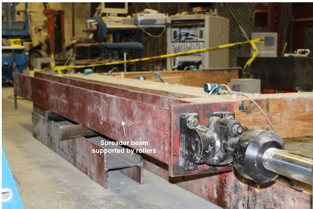
Fig. 3.6. DYWIDAG Anchor system securing actuator to the floor.
