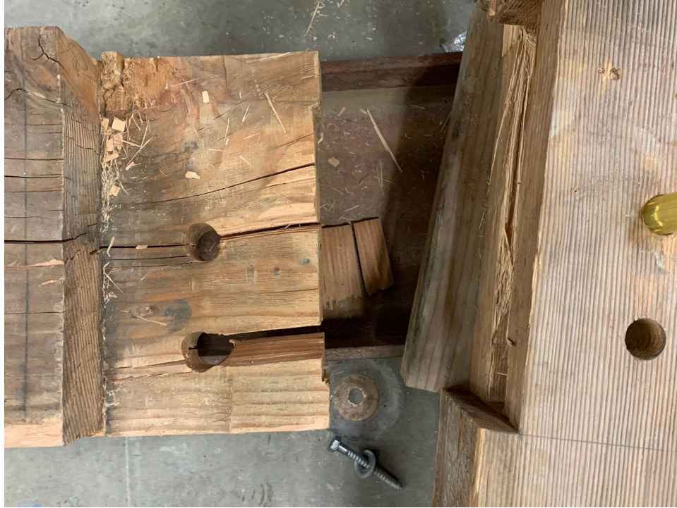
Fig. 3.31. Beam tenon from rehabilitated 2-peg frame displaying mode III m failure.
