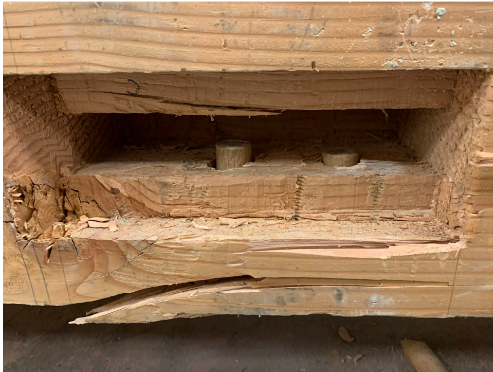
Fig. 3.32. Peg shear failure inside of post mortise from rehabilitated 2-peg frame.
