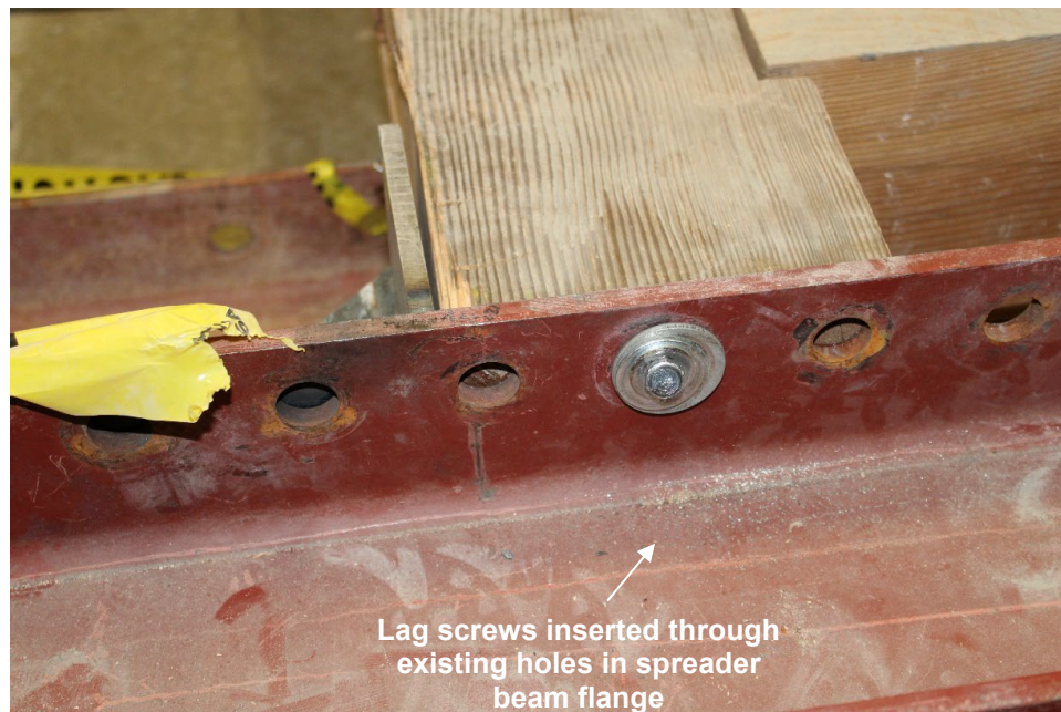
Fig. 3.10. Lag screw inserted into post to secure spreader beam.
