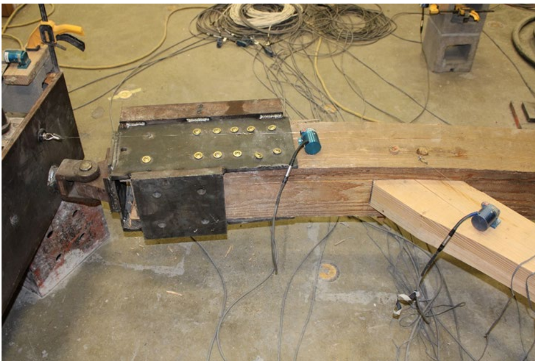
Fig. 3.21. Detail of left post footing experiencing flexure during the test.
