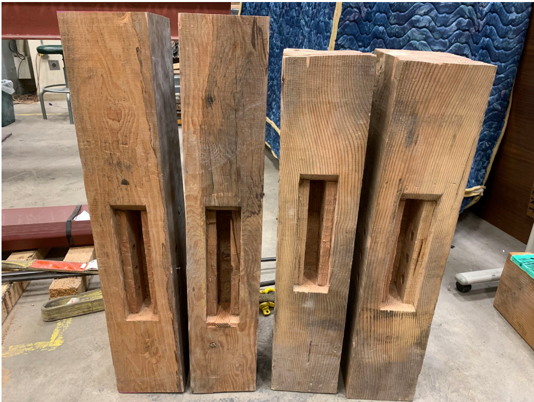
Fig. 4.1. Mortise specimens sourced from previously tested 3-peg frame.
