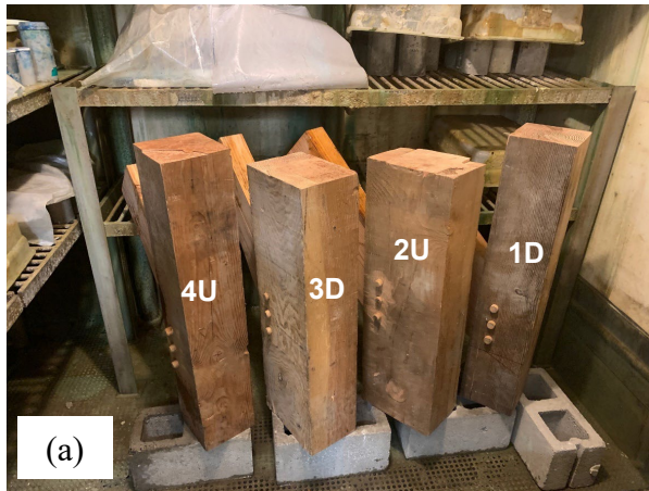
Fig. 4.4. Joint specimens: (a) at start of 6-month period, and (b) after 6-month period.
