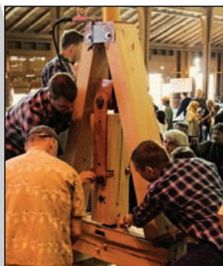
Fire Tower team removing failed wedged-dovetail thru tenon sample from tension tester at Asilomar.
