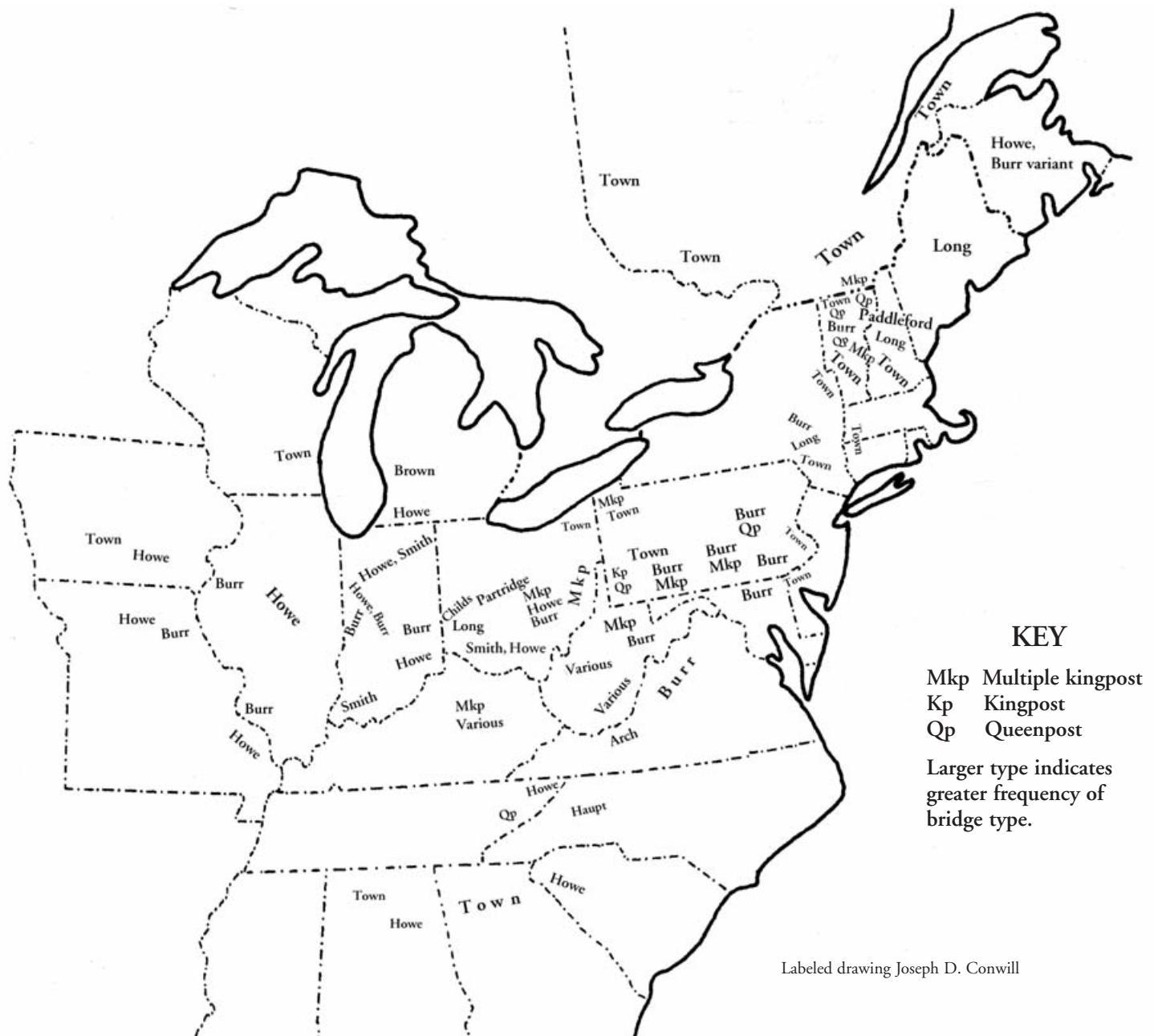
Fig. 17 Frequency distribution of covered bridge types in eastern US and Canada. Covered bridges in the West mainly use the Howe truss.
