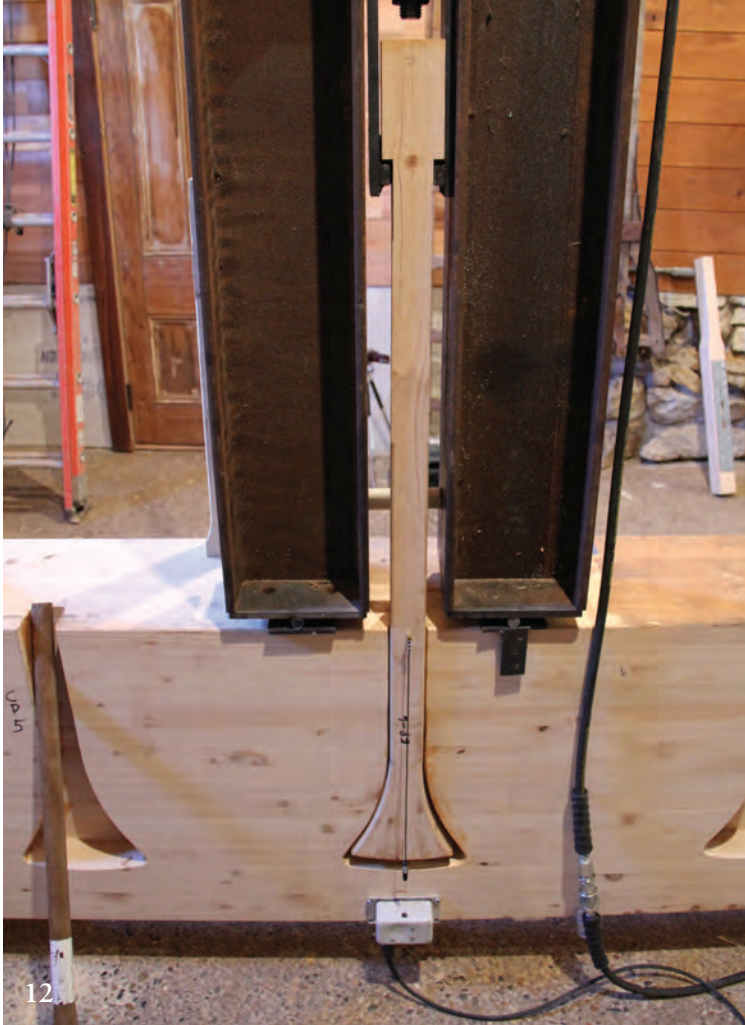
12 Full-scale mockup to test dovetail joint alone.
