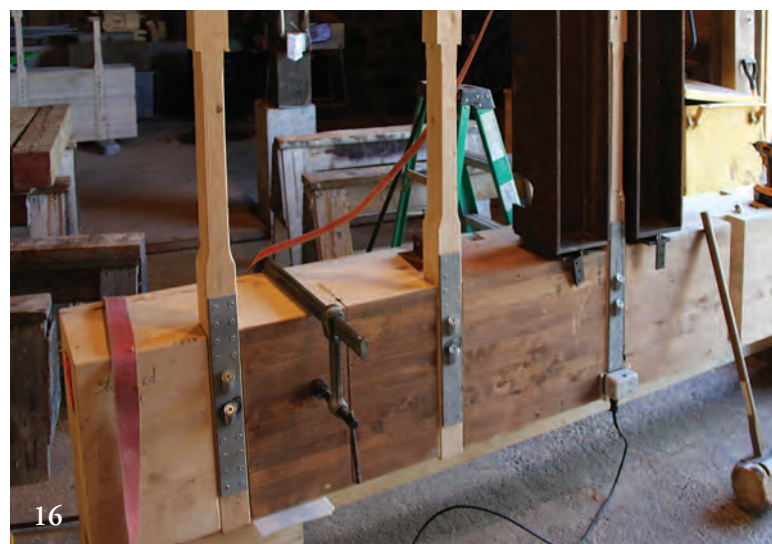
16 Tension-only connections similarly tested.
