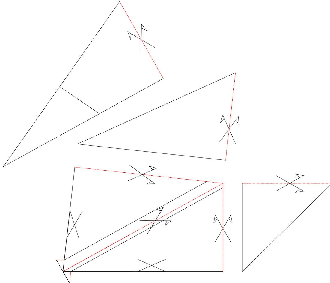
2-Where the line in step 1 intersect the hip gutter line, draw a line square through this point to intersect with both eave lines.
