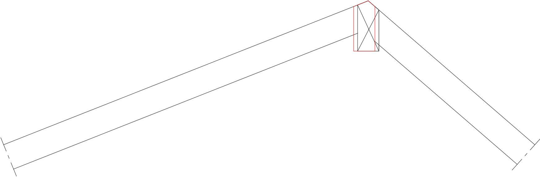
4-The hip is flush with one side of the roof or both sides with a backing angle.
