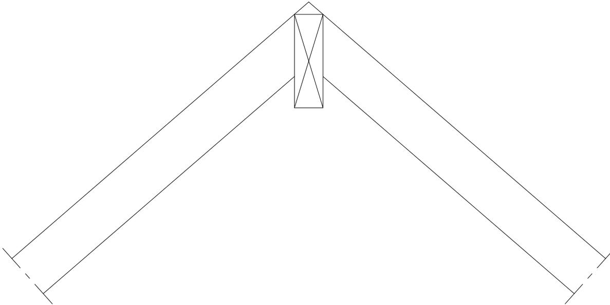
2-Centred with a backing angle. When the roof pitches are equal but the hip is wider than regular stick framing.
