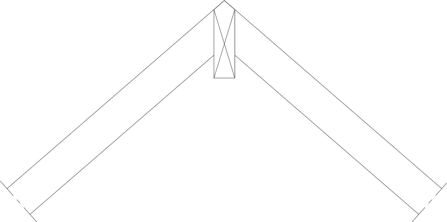
3-The hip is offset. When you have a main roof pitch different from the adjacent roof pitch. The reason to offset the hip is to save some material on the hip cross section.
