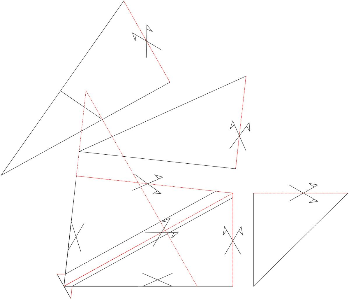
3-Take the length of the line drawn in step 1 and transfer it to the plan view on top of the hip centre line on either side of the where the line in step 2 intersects the hip in plan.
