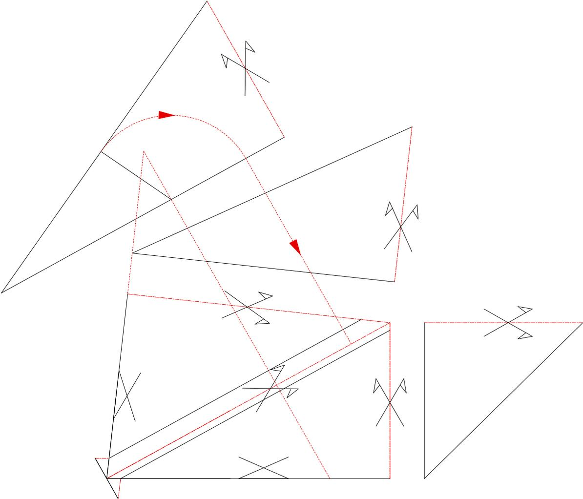
4-Connect the points obtained in step 2 and 3. This gives you the hip backing angle.
