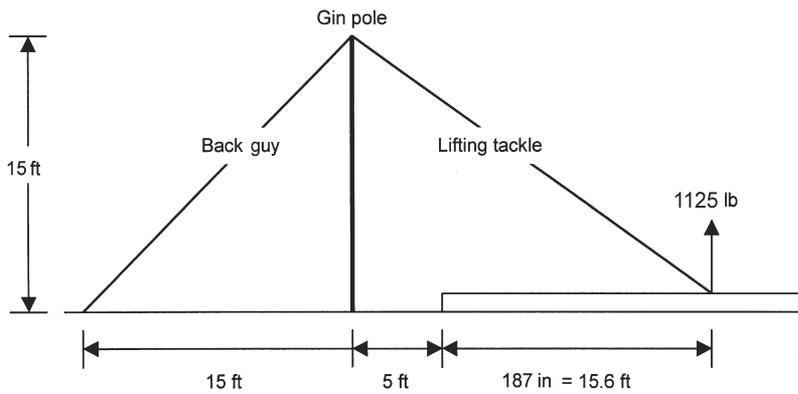
FIG. 6. GIN POLE LIFT DIAGRAM FOR CALCULATING LOADS.
