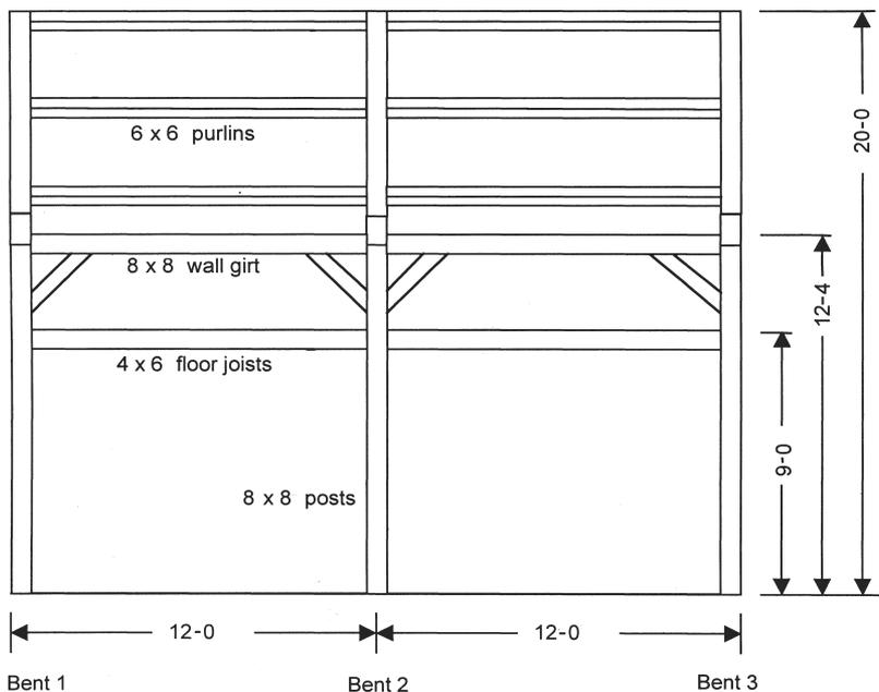
FIG. 3. ELEVATION OF A THREE-BENT MODEL FRAME.
