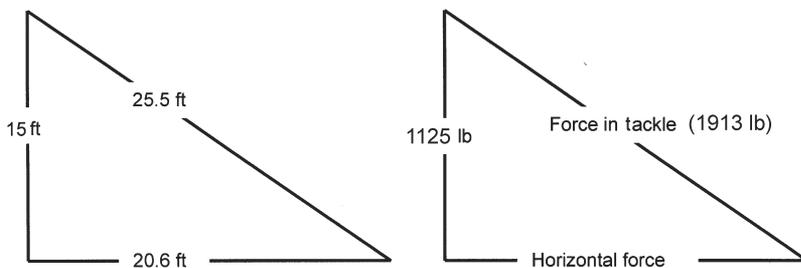
FIG. 7. CALCULATION BY METHOD OF SIMILAR TRIANGLES.
