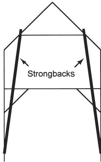
FIG. 9. STRONGBACKS FITTED TO ASSEMBLY TO PREVENT UNWANTED HINGING.
