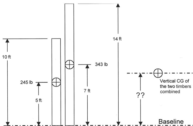
FIG. 4. COMBINED CENTERS OF GRAVITY FOR TWO TIMBERS.
