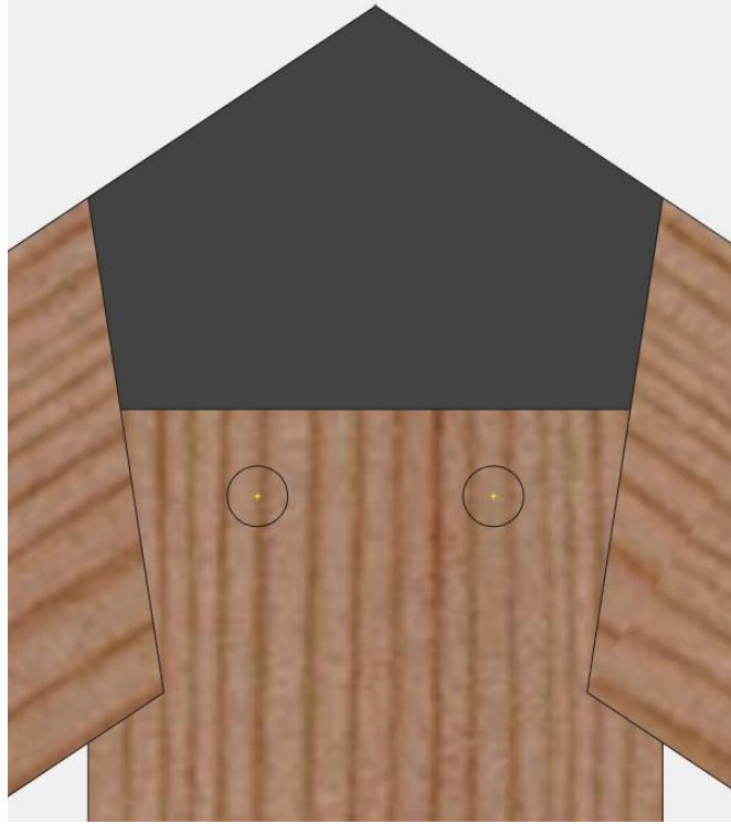
Figure C-2: Cross-section of a block shear plane in the KP of Peak Style A.
