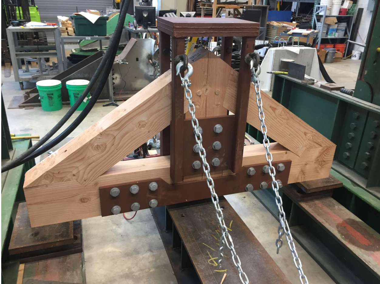
Figure 2-22: Truss in place in the UNH reaction frame (side shown is opposite the DIC painted side).
