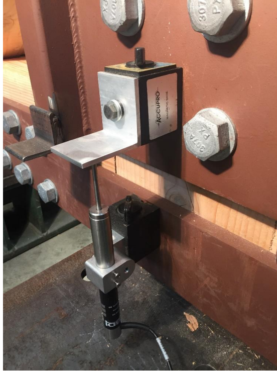
Figure 2-23: LVDT set up on steel testing frame using magnetic bases.
