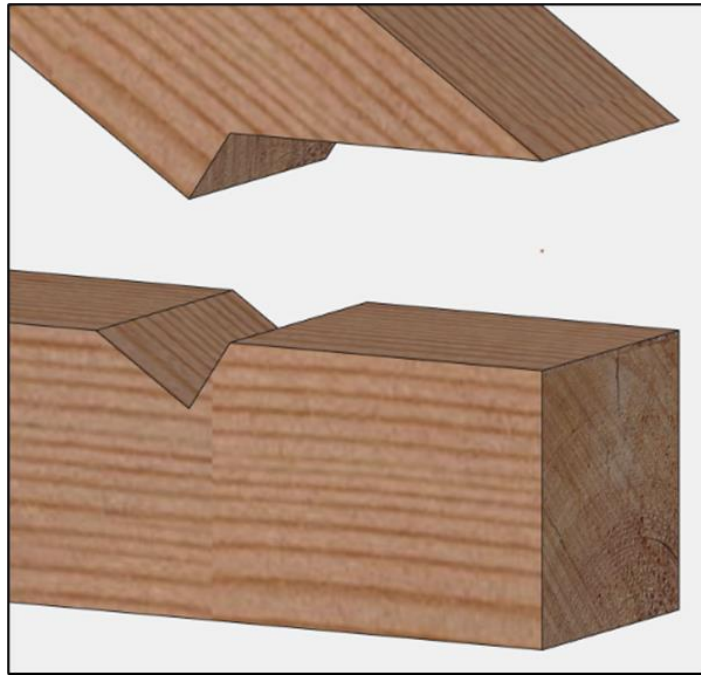
Figure 2-6: Birdsmouth shoulder at truss heel.
