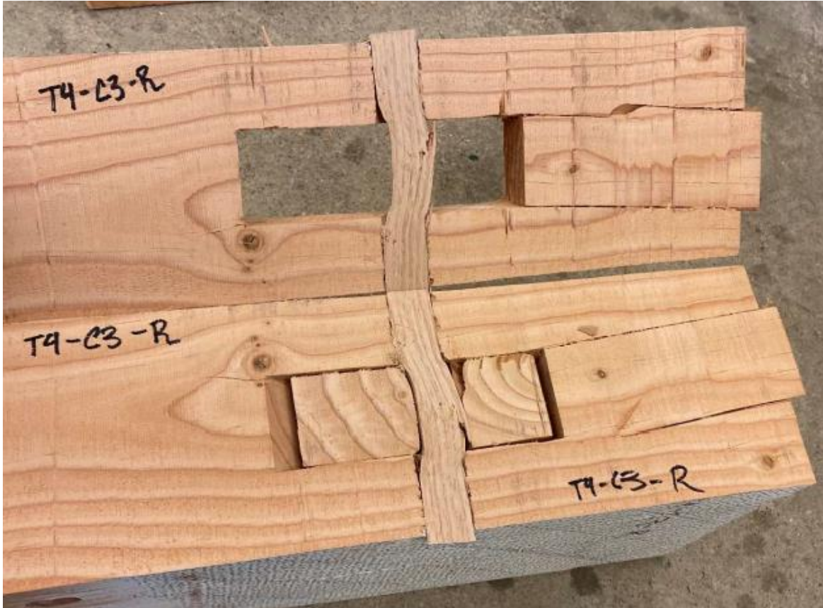
Figure 3-11: Yielded peg failure concurrent with block shear of the BC at Trial 4 Truss C3 Heel 2.
