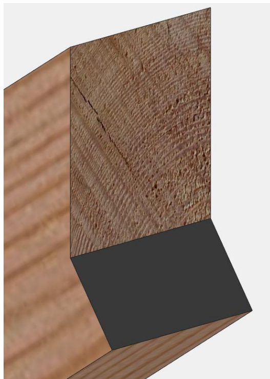
Figure C-3: Bearing area of TC shoulder for Peak Style C.
