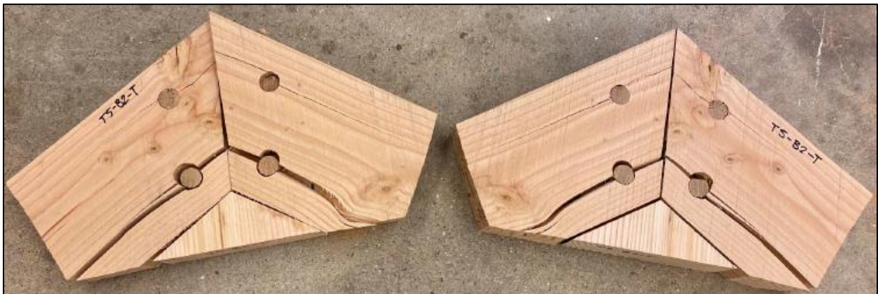
Figure 3-7: Cut view of Trial 5 Truss B2 crack formation at lower peg location.
