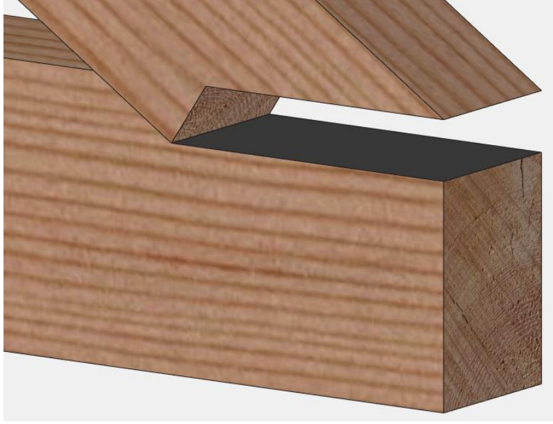
Figure C-6: Block shear plane of BC for Heel Style 1.
