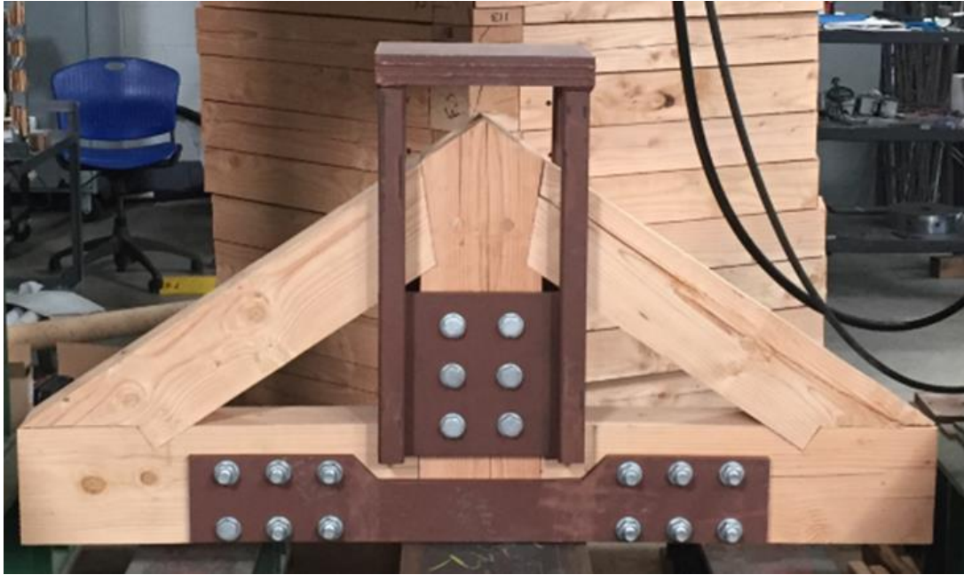
Figure 2-17: Steel loading frame and gusset plates shown on example Truss A1 specimen.
