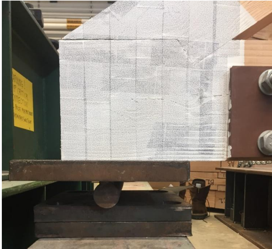
Figure 2-19: Truss heel support condition, showing roller support.
