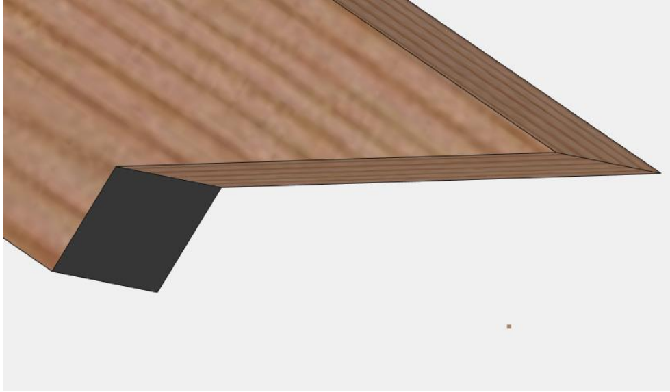
Figure C-5: Bearing area of TC shoulder for Heel Style 1.
