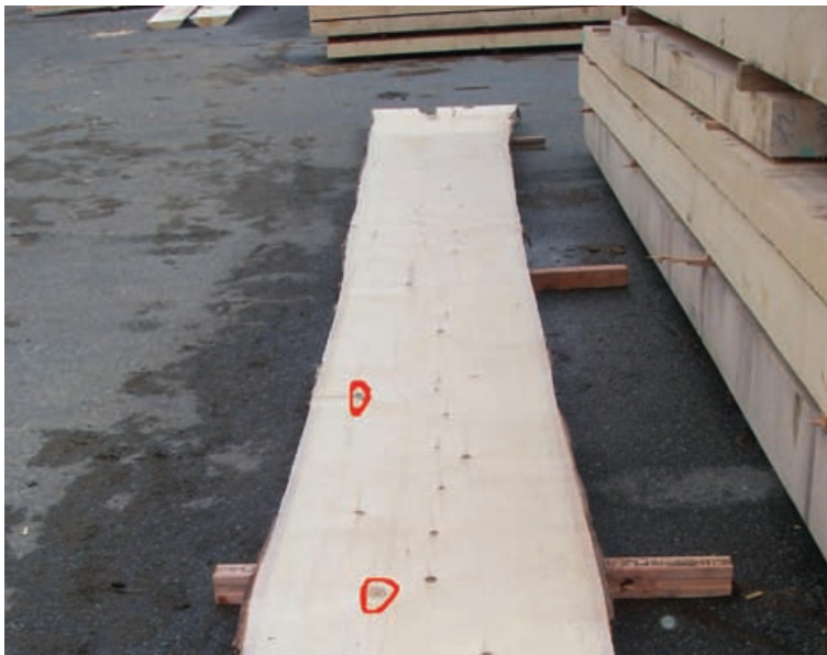
3 Almost D Clear yellow cedar. Nonconforming knots are circled.
