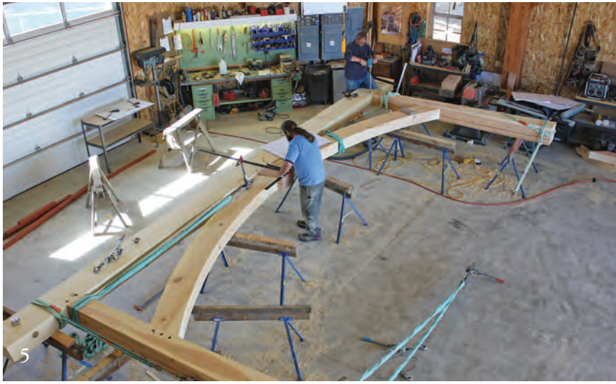
5, 6 Ponderosa pine performance pavilion in workshop and on dedication day in Sisters, Ore., built by Earthwood Timber Frame Homes of Oregon with the Kiwanis Club, both of Sisters. Above, Jason Soen fits “keystone” and Rod Zade drills for pegs. At right, Sisters Dance Troupe celebrates.
