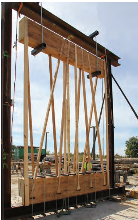
At left, full-scale tension test at Trillium Dell Timberworks, Knoxville, Ill., of 16-ft.-high mocked-up segment of hanging Port Orford cedar screen, part of walkway at new Writers Theatre in Glencoe, designed by Studio Gang, Chicago. Hydraulic jacks atop upper I-beam push up on steel tubes clamped to 12x24 upper chord. Battens 2x3, fastened at top with series of fully threaded screws, are wedged and spread at bottom to be captured in compound dovetail housings. Engineering by Joe Miller, Fire Tower Engineered Timber, Providence, R.I.
