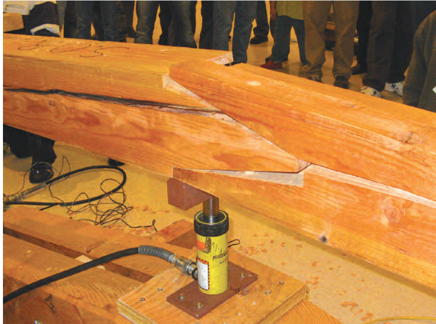
SOF (Saratoga or Bust) Scarf, Loyalist Timberframes. Code 2-VCS. Face-halved with sallyed and bridled butts. Moment transfer through bearing. Tension perpendicular to the grain failure as load pried joint apart.
