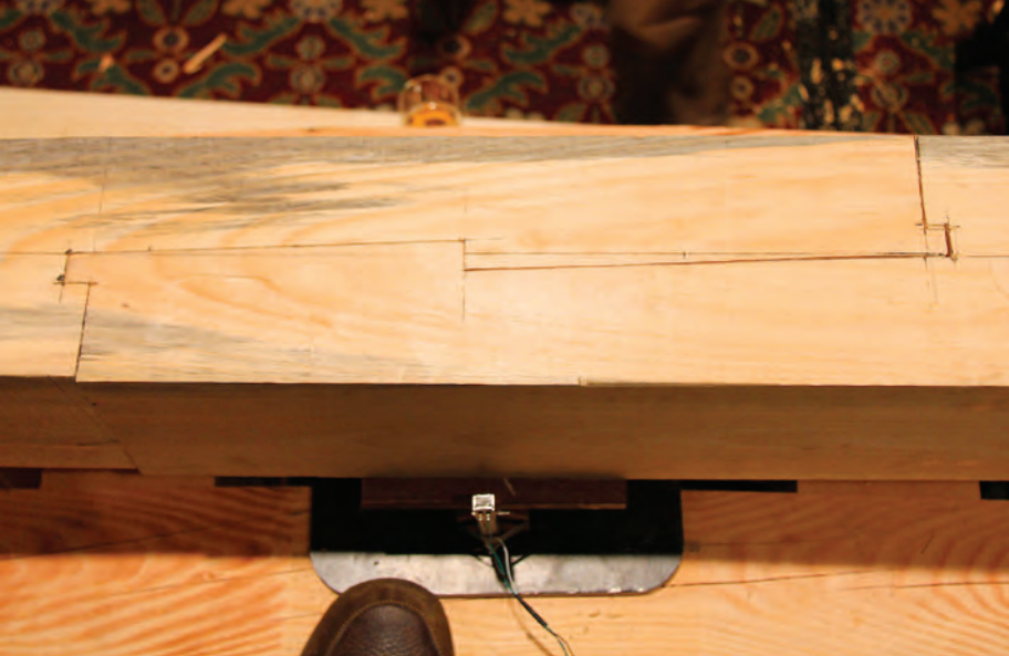
Okake Daisen, Adam Zgola. Code 15-VL. Face-halved, stop-splayed, tabled and bladed. Moment transfer through bearing alone. Block shear failure predominated with minor failure in tension perpendicular to grain. Inset shows detail of top view.
