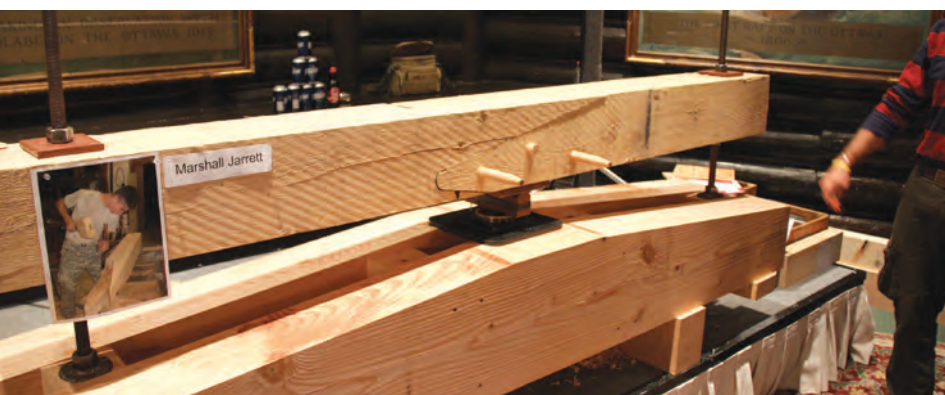
Jarrett Scarf, VMI. Code 9-VCSD. Variant on Bates. Face-halved with asymmetrical sallied butts and three edge pegs. Moment transfer through bearing and dowel shear. Failure in tension perpendicular to the grain (minimum dowel distress).
