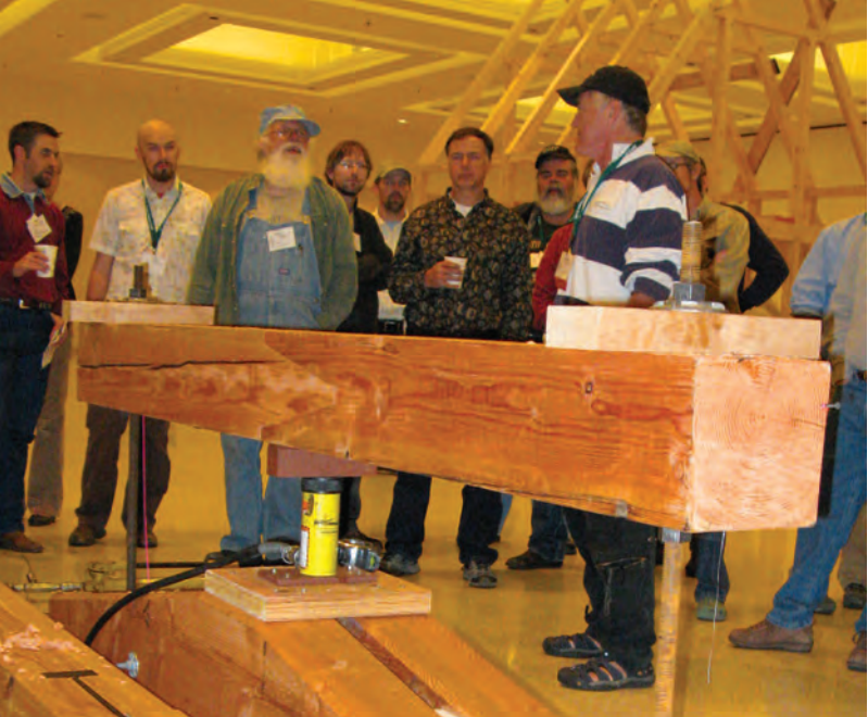
SOF (Saratoga or Bust) Scarf, Loyalist Timberframes. Code 2-VCS. Face-halved with sallyed and bridled butts. Moment transfer through bearing. Tension perpendicular to the grain failure as load pried joint apart.
