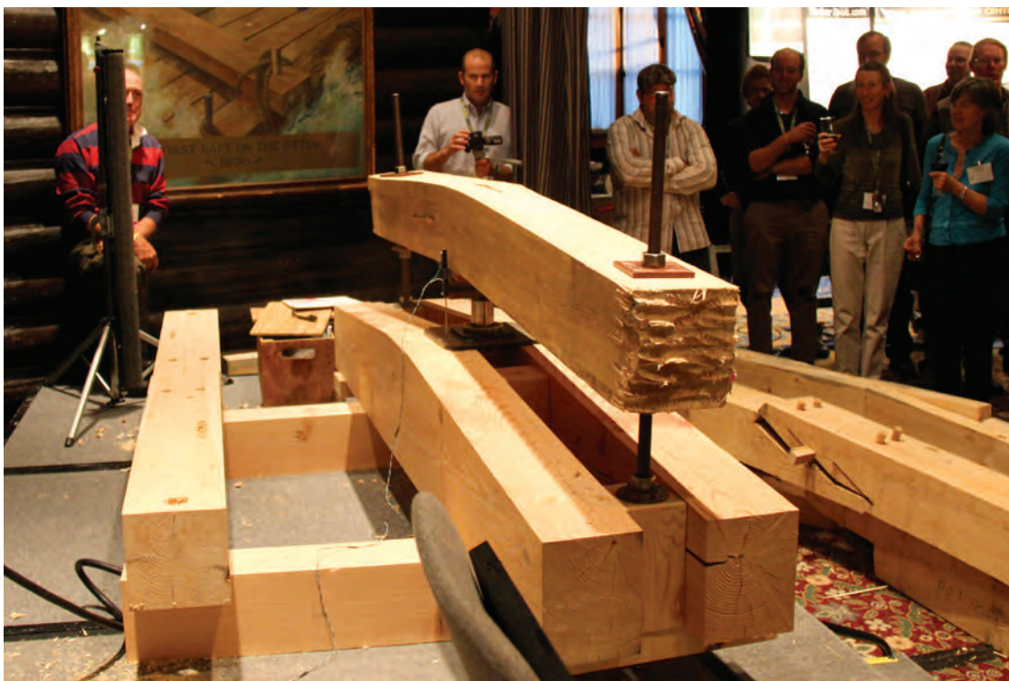
Hamlet Hemlock Solid-Sawn Beam, Hamlet Heavy Timberworks. Code 13-MN. Mother Nature's entry. Classic modulus of rupture failure, at 33,840 lbs. Test beam was parted from longer one with drill and auger bit, under desperate conditions.
