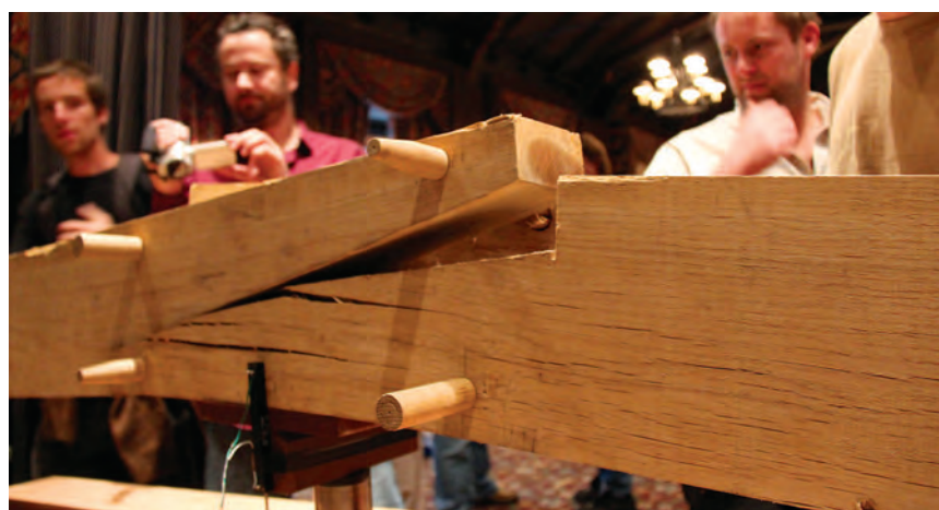
Peck Scarf, VMI. Code 10-VLSD. Face-halved scissor with four edge pegs. Moment transfer through bearing and dowel shear. Failure first through dowels followed by failure in tension perpendicular to grain.
