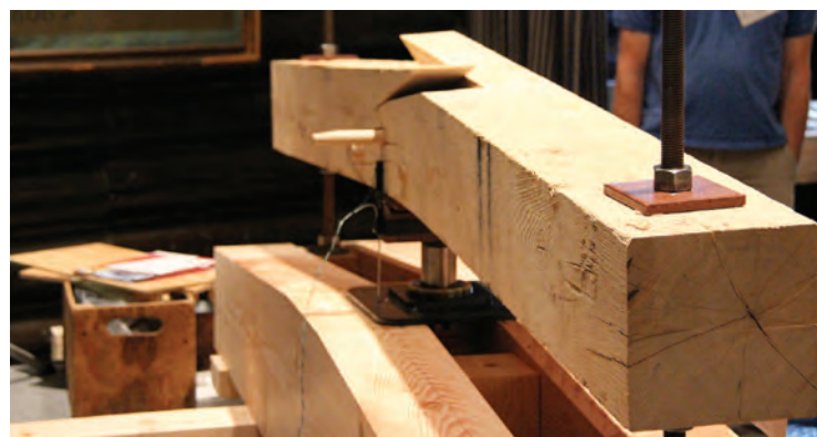
Jarrett Scarf, VMI. Code 9-VCSD. Variant on Bates. Face-halved with asymmetrical sallied butts and three edge pegs. Moment transfer through bearing and dowel shear. Failure in tension perpendicular to the grain (minimum dowel distress).
