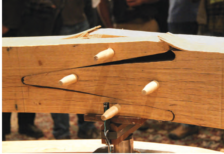
Bates Scarf, Virginia Military Institute (VMI). Code 8-VCSD. Face-halved with sallied butts and four edge pegs. Moment transfer in bearing and dowel shear. Failure in tension perpendicular to grain and dowel shear.
