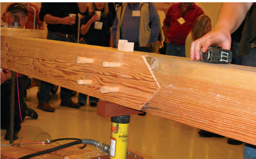
Below, Diamond Dove Scarf, Timberpeg. Code 4-CVLD. Face-halved and keyed with lapped sallyed butts and four edge pegs. Moment transfer through squinted bearing surfaces and dowels. Block shear failure.
