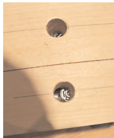
Okake Daisen, Adam Zgola. Code 15-VL. Face-halved, stop-splayed, tabled and bladed. Moment transfer through bearing alone. Block shear failure predominated with minor failure in tension perpendicular to grain. Inset shows detail of top view.
