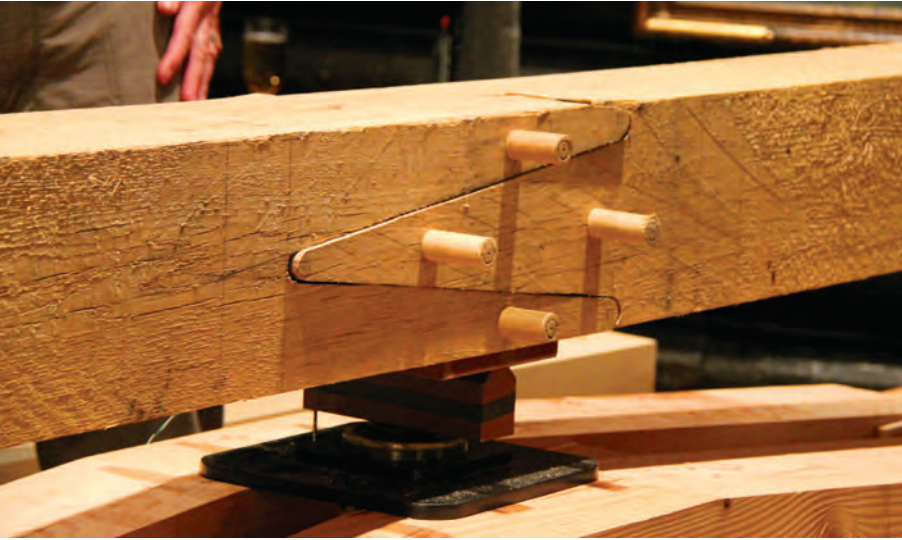
Bates Scarf, Virginia Military Institute (VMI). Code 8-VCSD. Face-halved with sallied butts and four edge pegs. Moment transfer in bearing and dowel shear. Failure in tension perpendicular to grain and dowel shear.
