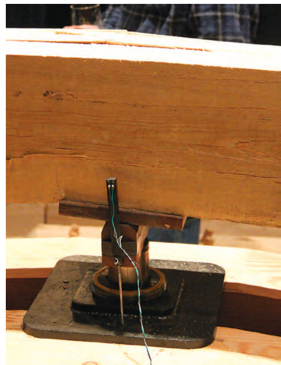
Hamlet Hemlock Solid-Sawn Beam, Hamlet Heavy Timberworks. Code 13-MN. Mother Nature's entry. Classic modulus of rupture failure, at 33,840 lbs. Test beam was parted from longer one with drill and auger bit, under desperate conditions.
