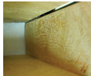
Figs. 21–22. At left, side-grain crushing in sloped white oak shear keys. At right, end-grain interpenetration of PSL key in poplar housing.
