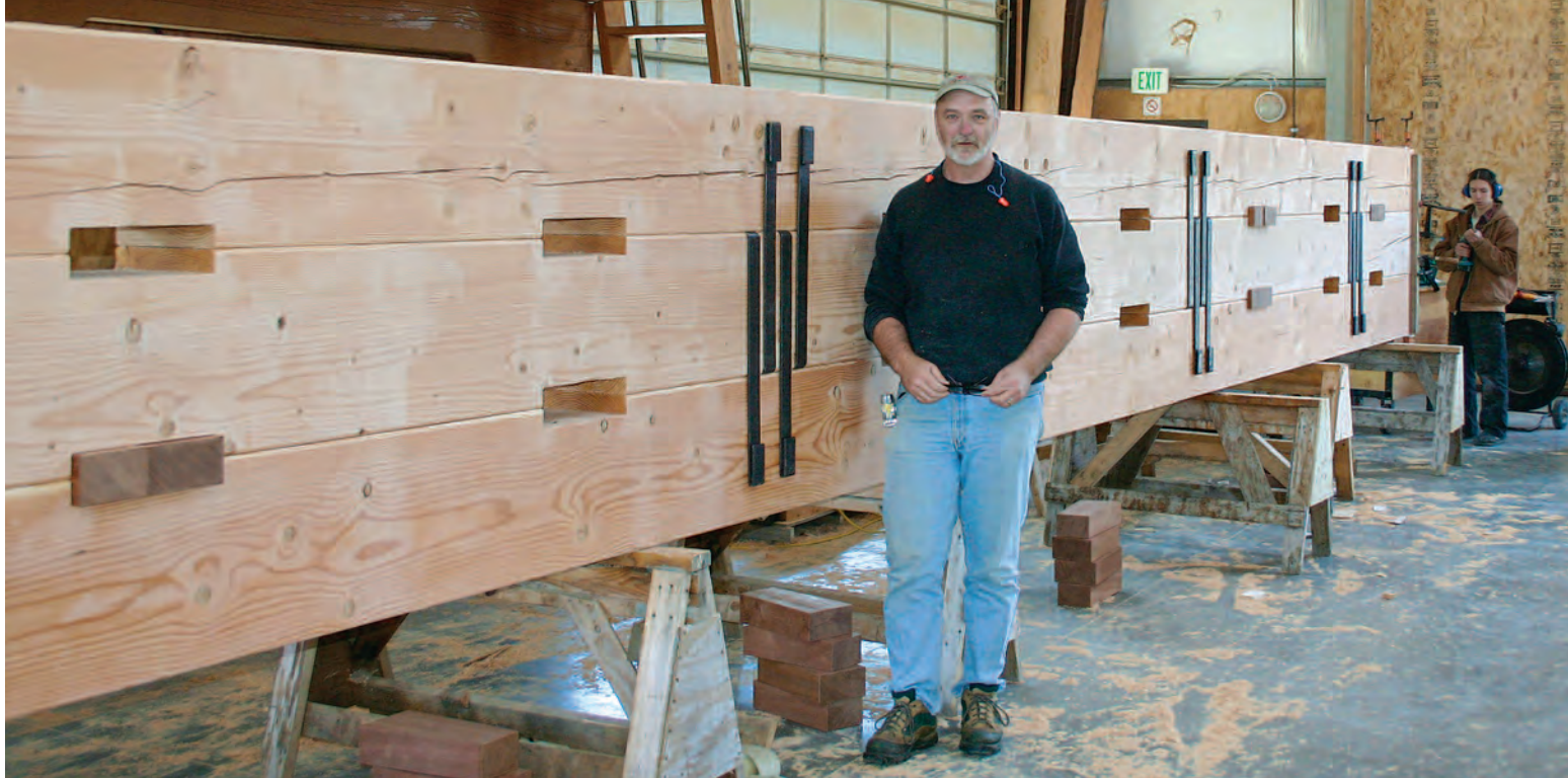
Fig. 1. Mechanically laminated beams handle unusual loads, preserve beauty of natural timber and offer decorative possibilities. Folding wedges to develop shear resistance at beam interfaces are seen partly installed and stacked on shop floor at Cascade Joinery, Bellingham, Washington. Iron straps remain to be completed to cinch assembled beam against being driven apart by reaction to wedging.
