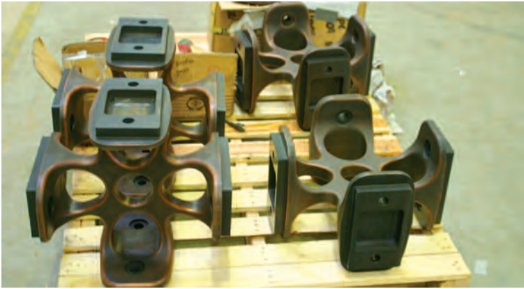
Fig. 16. At Wawona, through-bolted cast-aluminum keys electroplated with copper and bronzed fit rectangular housings. Bolt heads lie flush.
