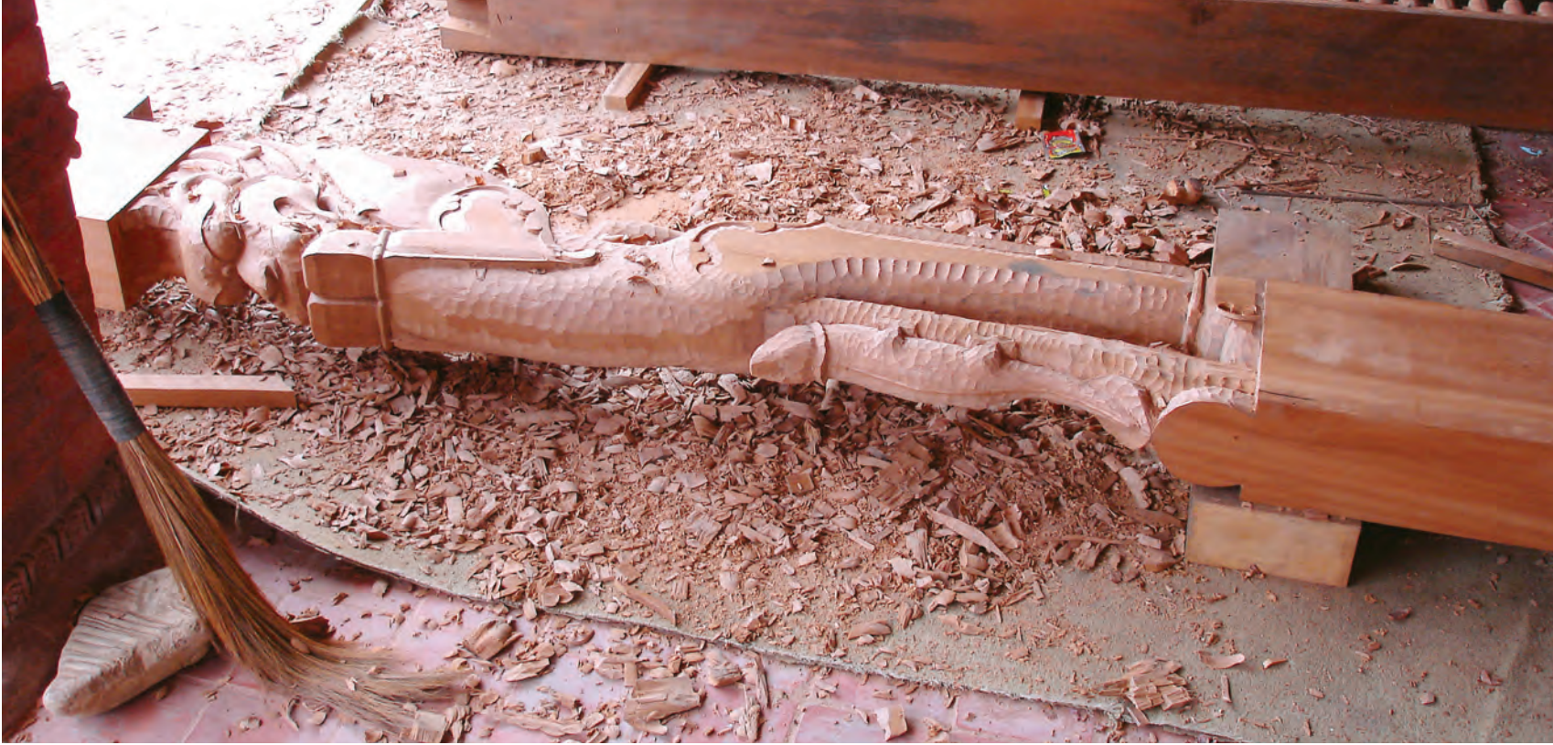
Fig. 20. Woodcarving, a defining art form of Nepal, contributes to national consciousness. Massive strut shown for new Pokhara temple will support one corner of large lower chhana (overhanging roof). Struts will carry jetty plates and rafters secured with square pegs. Note sharpening stone, worn in for gouges, in left foreground.
