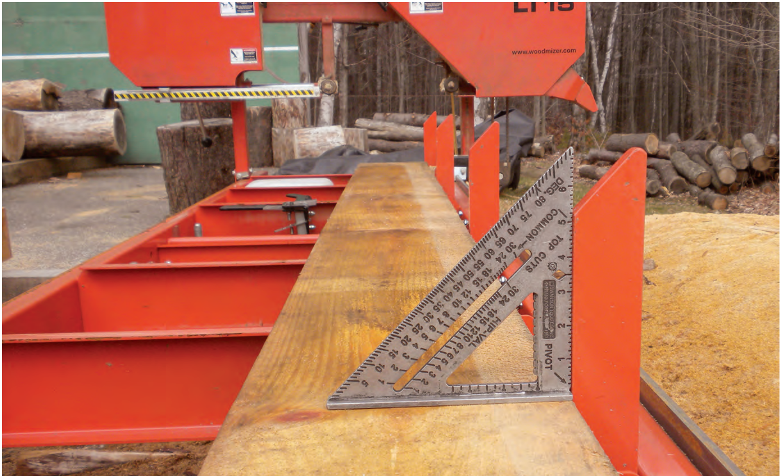
Fig. 2. Adjustable side supports should be squared to trued-up mill bed.
