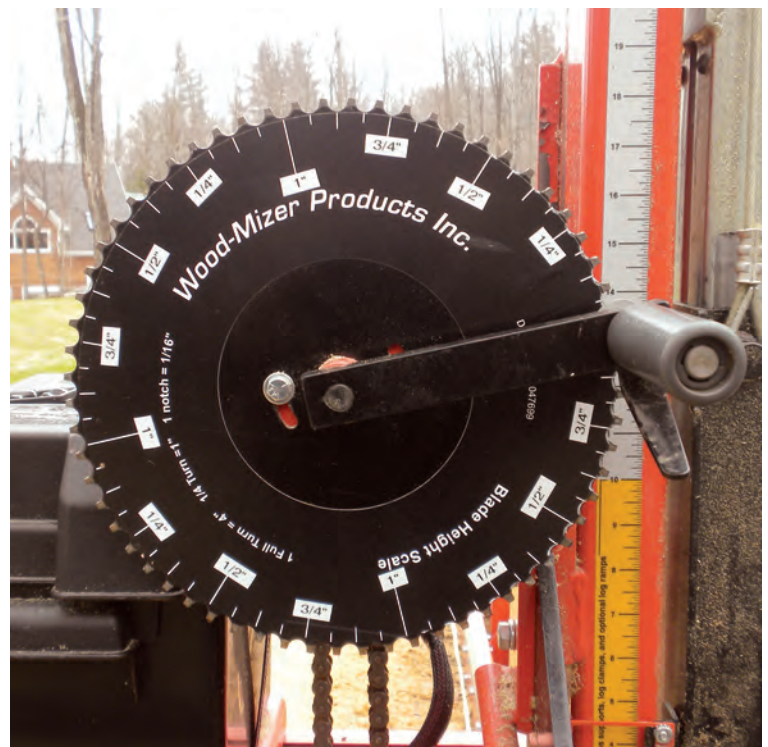
Fig. 3. Each notch of the crank wheel raises or lowers the blade by \frac{1}{16} in. Lock release shown below end of crank handle.
