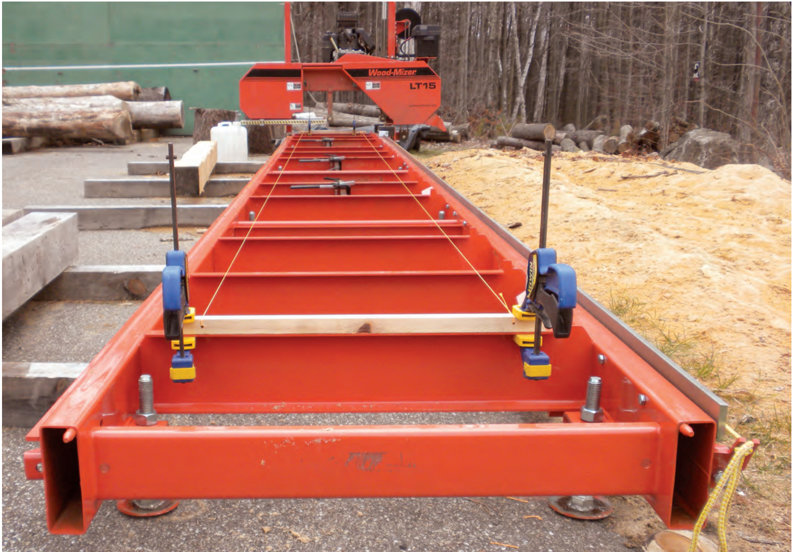
Fig. 1. A simple jig holds strings above the bed rails to aid in truing the mill. Clamps attached to crossrails at far end of mill are log dogs.
