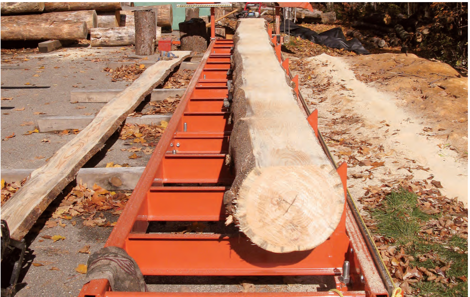
Fig. 6. The cant after first cut. Flitch on left.
