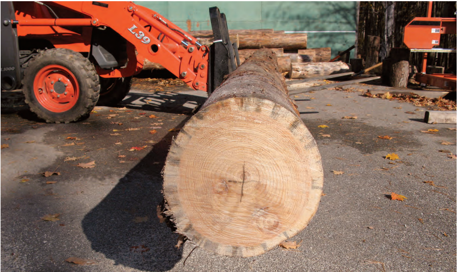
Fig. 5. White pine log on forks, a good time to clean the log, mark centers and check for crook.
