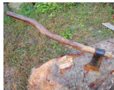
Fig. 2. Nepali axe with forged round eye and sharply curved bit, apparently hafted for hewing.
