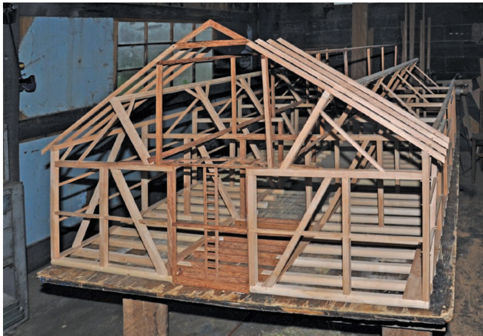
10 Model of split barn commissioned by authors and built by Andy Ebersol of Airville, Pennsylvania, using Michigan beech (from coauthor's family farm) for original barn timbers and contrasting Brazilian cherry for infill pieces. Note horizontal truss.
