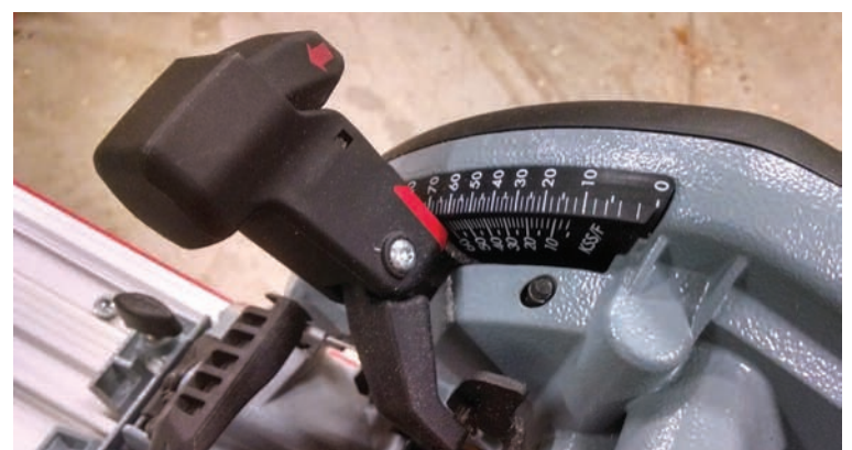
5 Squeeze-operated depth-setting lever and scales off and on track.
