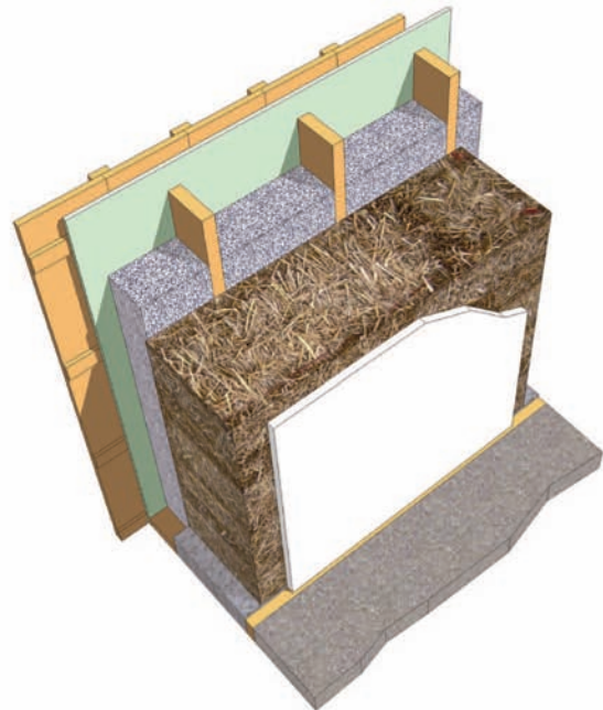
6 New Frameworks system with cellulose insulated 2x6 wall to outside of 14-in. strawbale wall, omits wall timbers.
