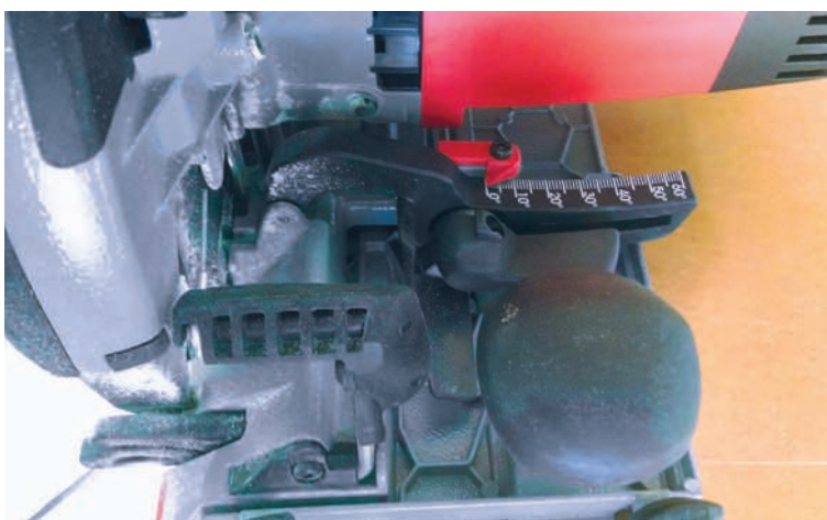
4 Bevel lock and scale behind knob, guard-retracting lever to left.
