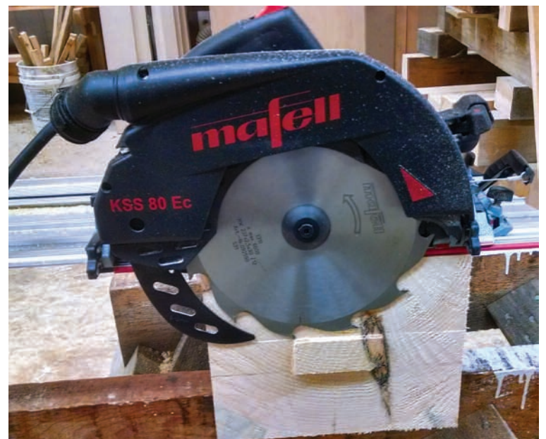
3 In-track depth of cut is 3\frac{3}{4} in. Riving knife descends with blade to keep kerf open behind blade. Dust chute rotates and accepts hose.
