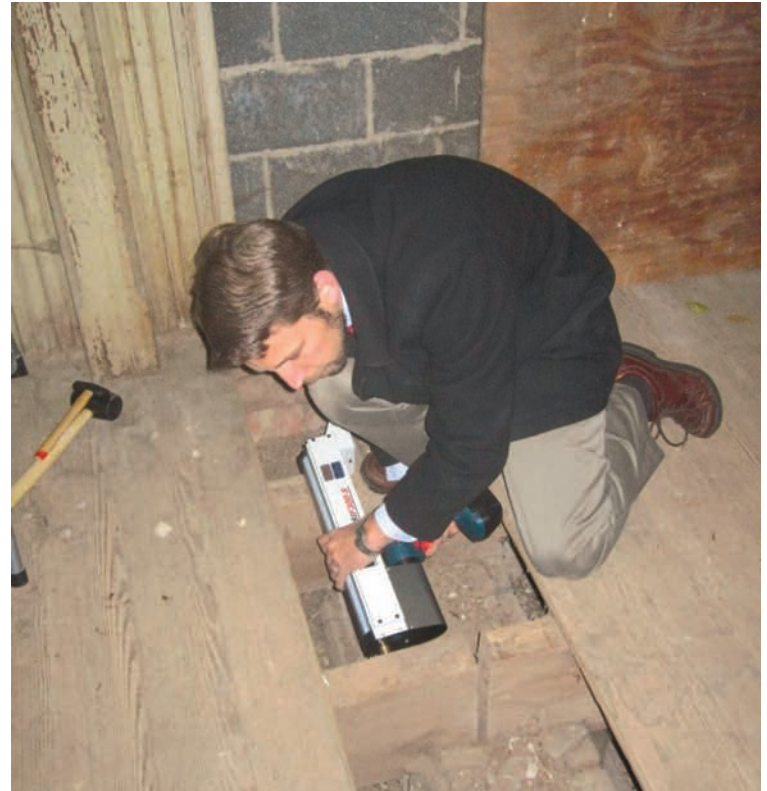
9 IML Resistograph being used by author to assess a joist at Union Church (ca. 1819) in Falmouth, Virginia.
